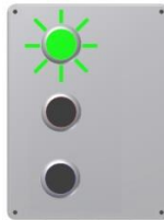
Flashing Green Machine Stopping
